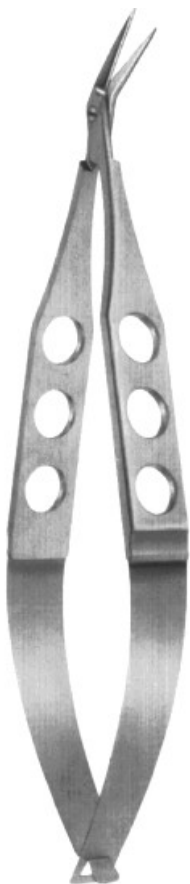
77-671-11 Castroviejo Keratoplasty Scissor Angled to Side, Blunt Tips 14 mm Long Blades With Max. 9 mm Cutting Edge Overall Length 11.5 cm (4 ½")
