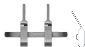
23-027-17 Biemer-Mueller Approximator 17 mm, Straight, Narrow Opening : 5 mm Jaw Length : 9 mm Closing Pressure : 25 - 30 gr
