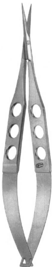
77-690-11 Fine Micro Scissor Straight, Sharp Tips 17 mm Long Blades With Max. 9 mm Cutting Edge Overall Length 11.5 cm (4 ½")
